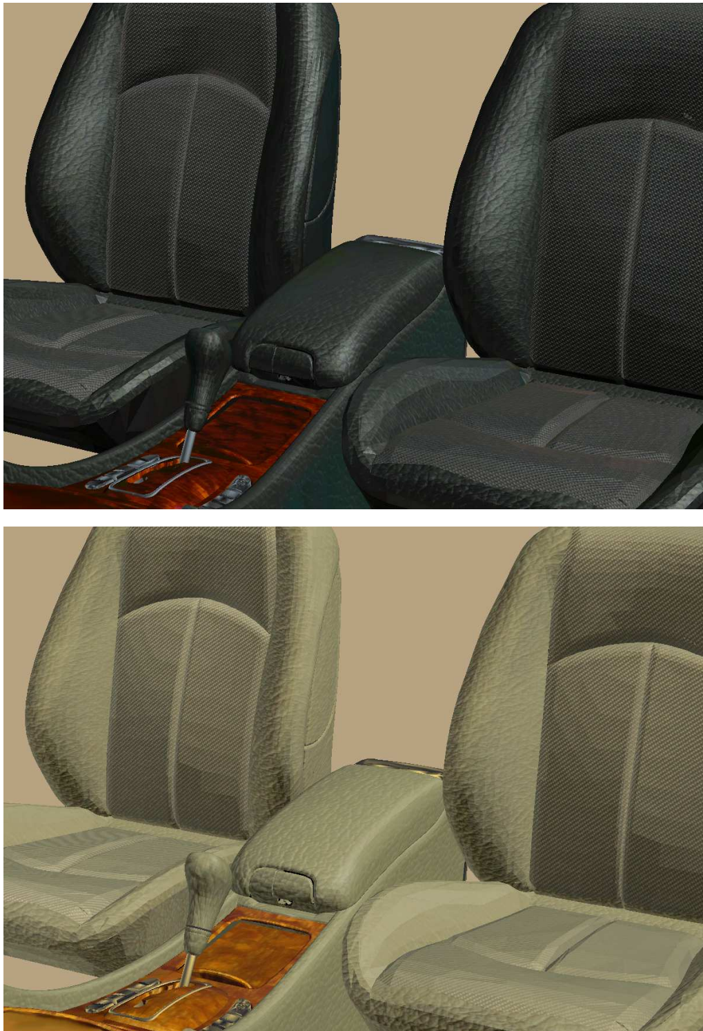
Figure 8.18: Two partial examples of car interior modelling (Mercedes-Class C). Images illustrate seven different materials: wood01 , wood02 , foil01 , foil02 , fabric01 , fabric02 , leather02 approximated by means of proposed PLM-C BTF model.
