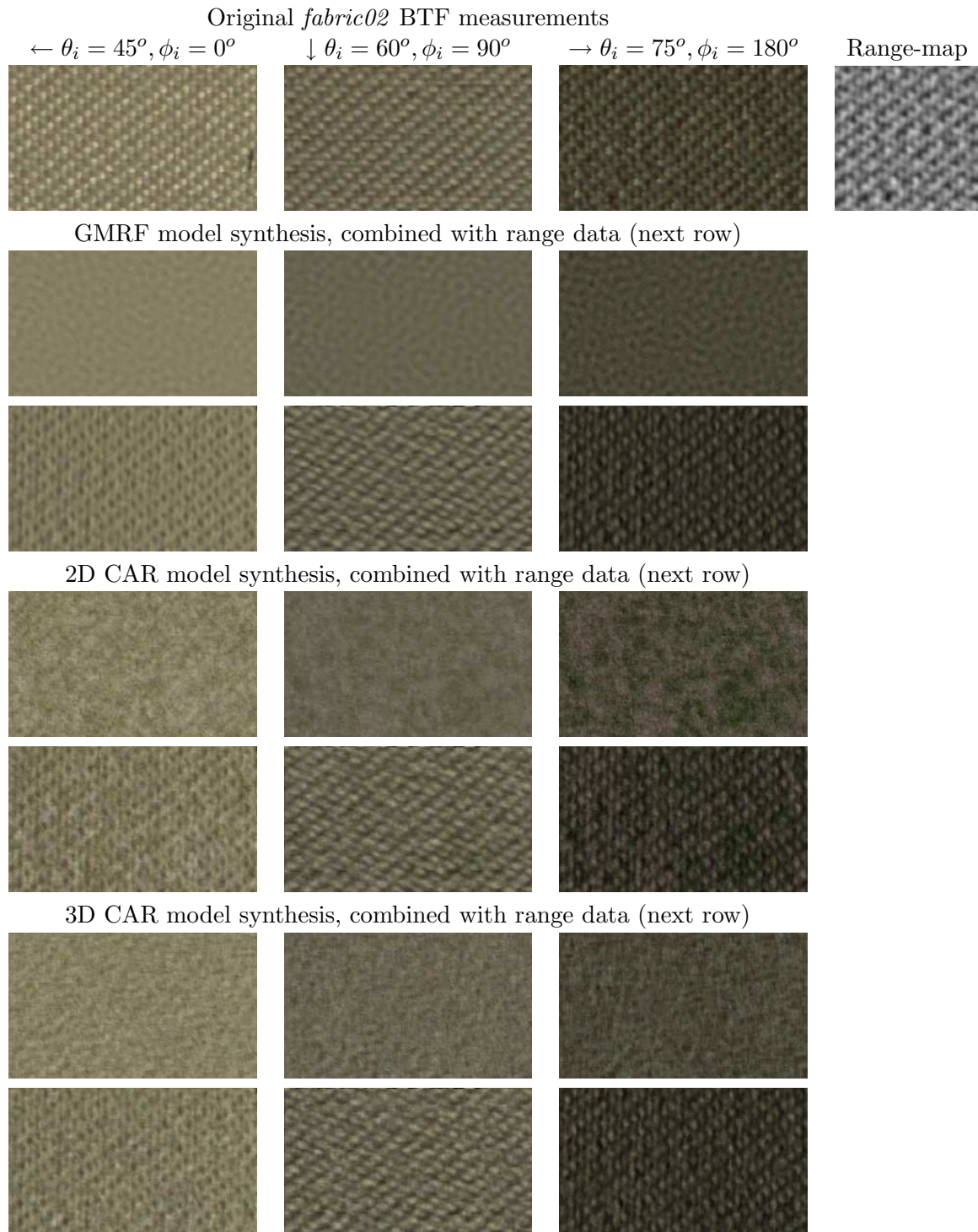
Figure 7.7: Fabric02 synthesised BTF images obtained using proposed probabilistic BTF models: GMRF, 2D CAR and 3D CAR respectively compared with corresponding raw BTF measurements for three distinct illumination directions. Range data were introduced into the models by means of displacement mapping.
