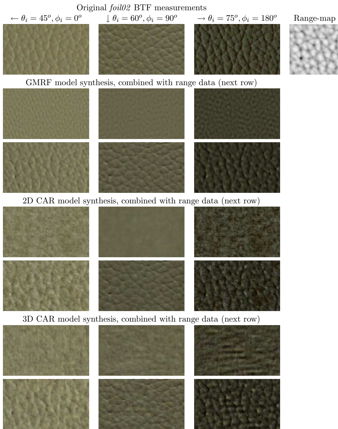
Figure 7.8: Foil02 synthesised BTF images obtained using proposed probabilistic BTF models: GMRF, 2D CAR and 3D CAR respectively compared with corresponding raw BTF measurements for three distinct illumination directions. Range data were introduced into the models by means of displacement mapping.
