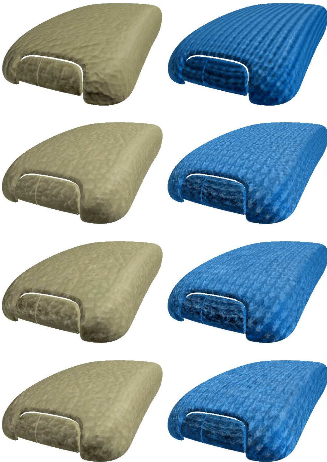
Figure 7.16: Original BTF on car armrest for leather02 and wool materials (first rows) compared with results of GMRF, 2D CAR and 3D CAR BTF models respectively. Regular surface structure introduced by means of bump mapping.
