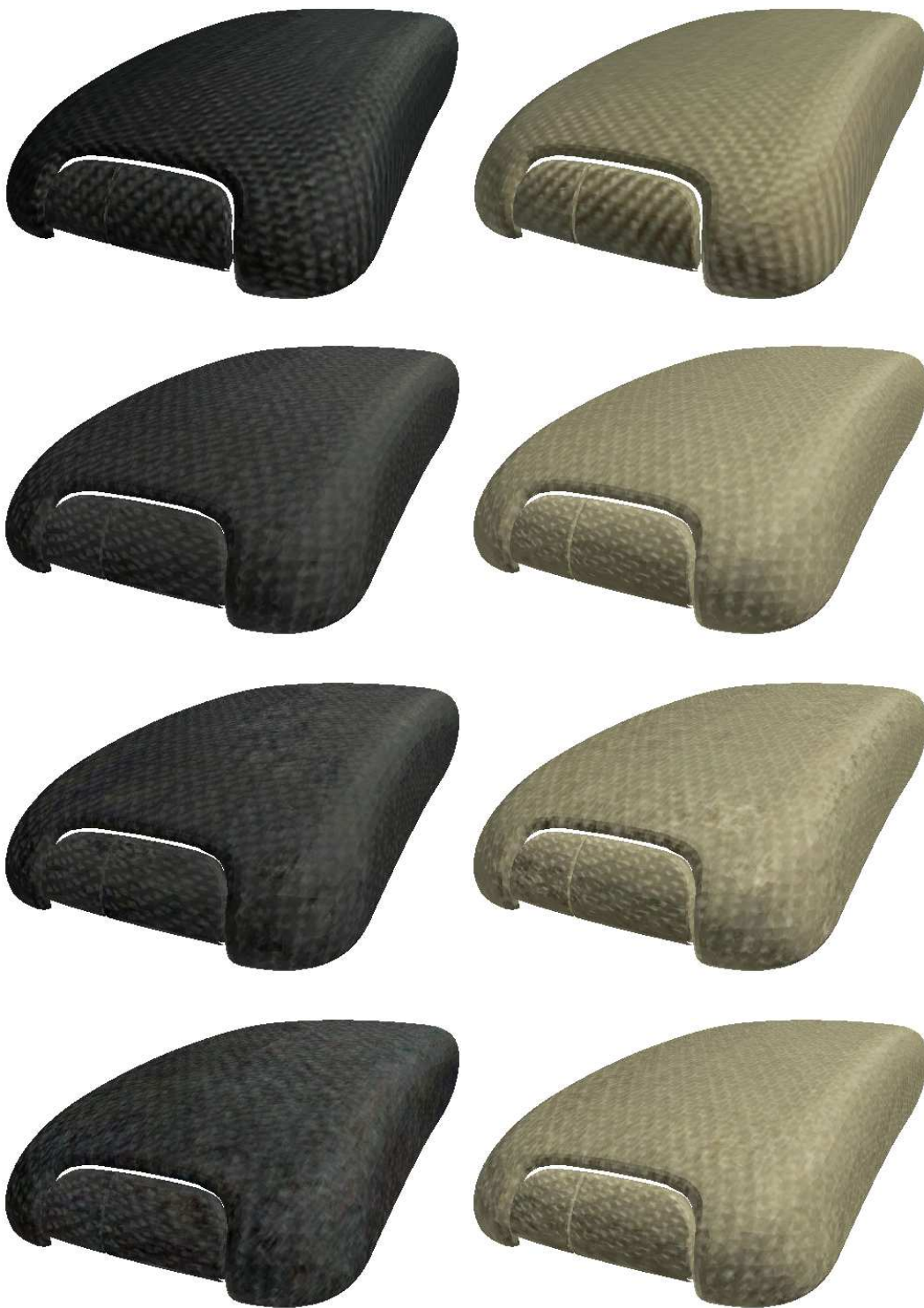
Figure 7.14: Original BTF on car armrest for fabric01 and fabric02 materials (first rows) compared with results of GMRF, 2D CAR and 3D CAR BTF models respectively. Regular surface structure introduced by means of bump mapping.
